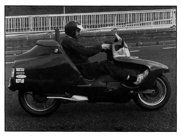
justify fitting the higher final drive gearing from the Moto Guzzi 'Convetf range. At a minor cost in initial acceleration this allowed relaxed high speed cruising with excellent fuel economy.
